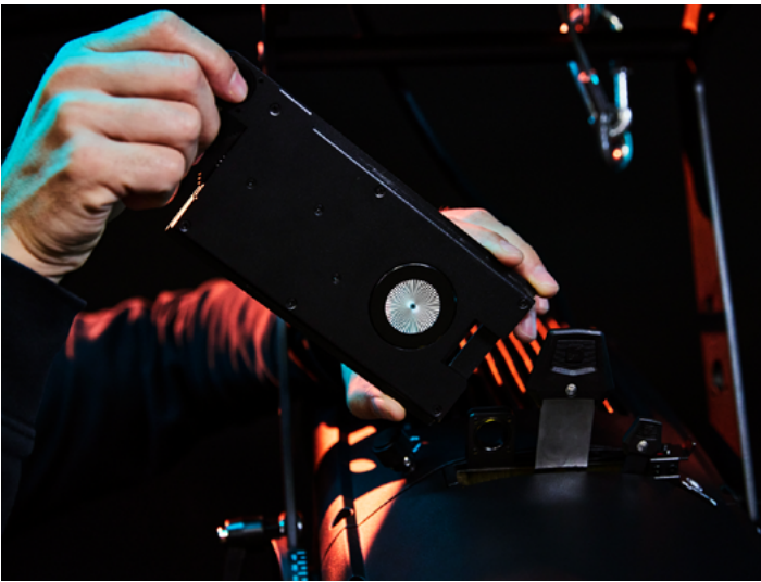
Orientation Reminder: Gobos are always inserted up-side down and mirrored. Watch for the correct coating direction – coated side facing away from the lamp.
